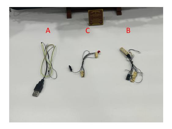
Stick the led strip from lighting part A under the front side of the ship Before that remove the ship from the rack and detach the shown black part \*Note: the end in the red circle should be the USB plug, which means the USB should be at the rear side of the ship
