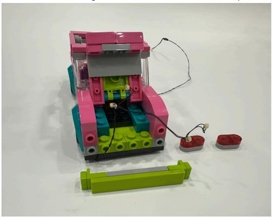
Insert the led bulbs inside the hole of the grey plates from behind
