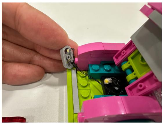
Get the led through the hole, put the grey plate back on the car and press the led bulbs inside the hole
