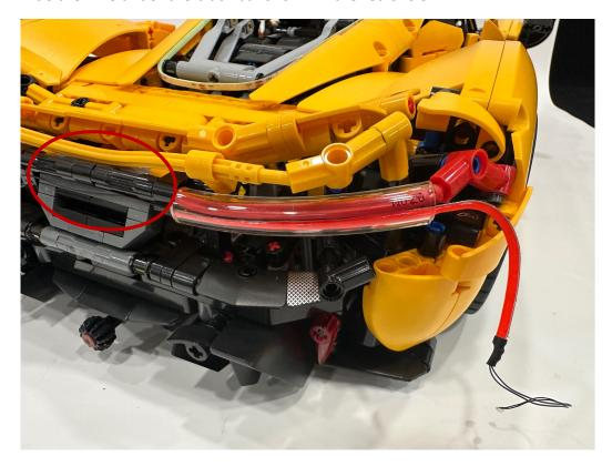
Then assemble the led strip with the tube by the same way as the other side
