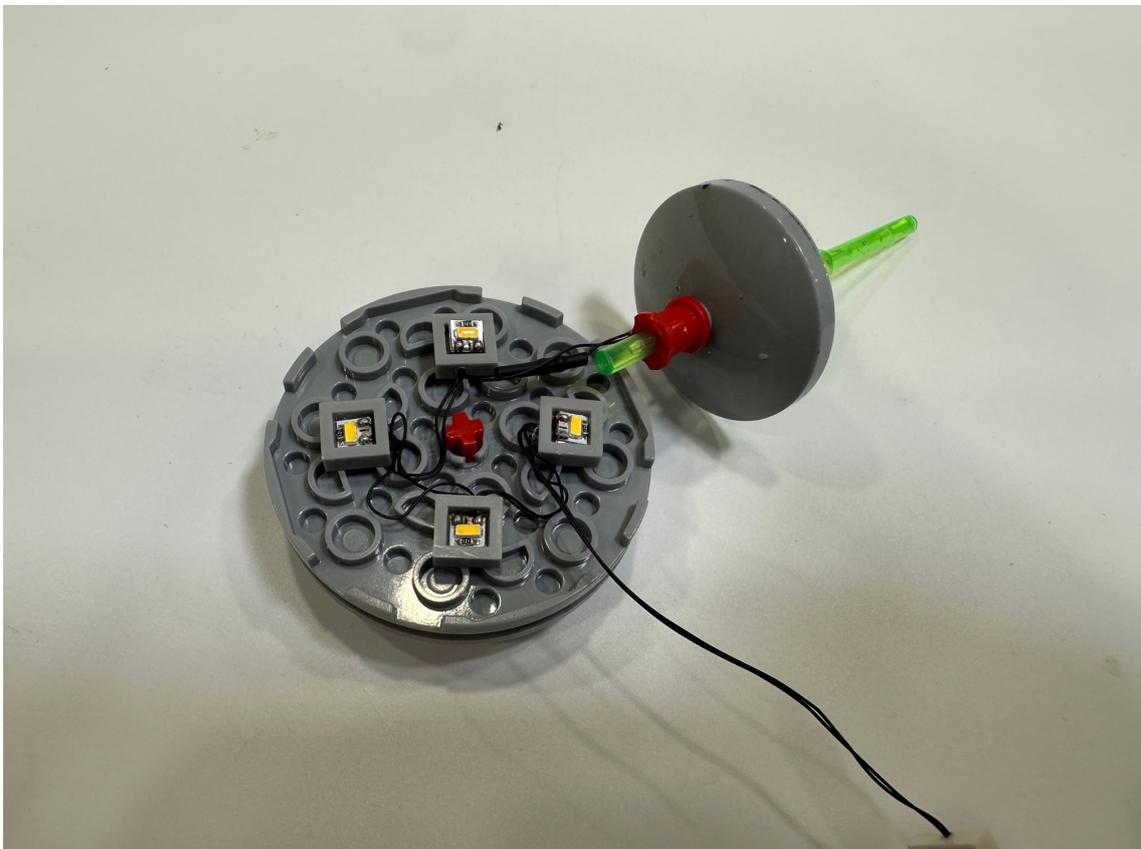
Restore the top and take the shown parts out to move the remain parts down to the bottom
