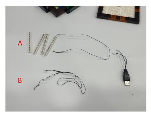
Assemble the lighting part A to under the top of the model
