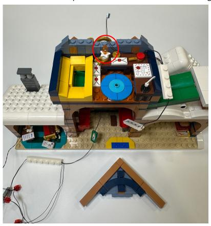
Stick the led plate at the shown spot, restore the wall and be careful the wire has to be placed in between the studs
