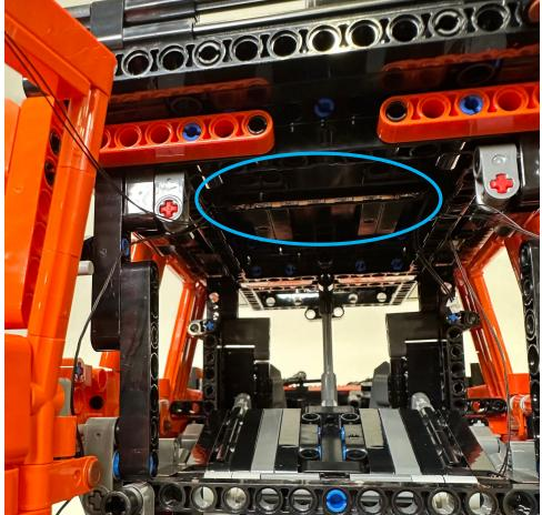
Get the wire with connector through to the bottom of the car
