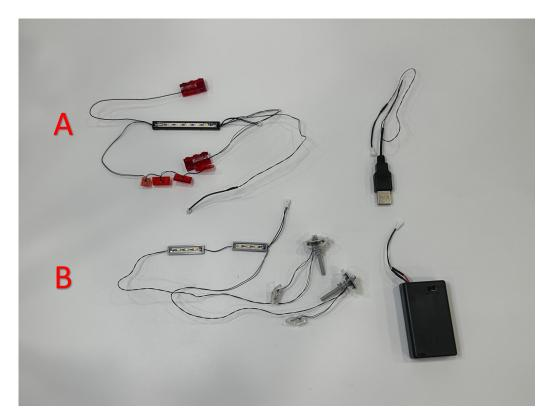
Take lighting parts A to assemble on the rear of the car Firstly take away the rear lights, keep the orange 1x3 tiles and put them on the lighting parts as shown
