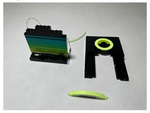
Move the long led strip to the front, place the wire in between the stud then restore the top half of the slide but don't close it tight yet
