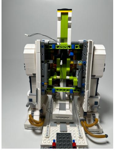
Then put the USB cable back behind the model and move the longer connector to the head position
