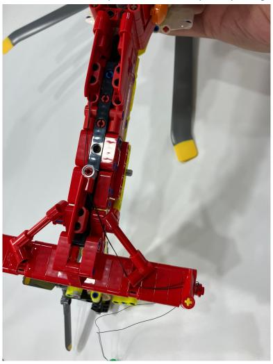
Move the green lighting round plate to the other side and assemble it Hide as many as the wires underneath the wing to make them invisible from the top
