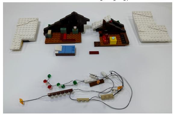
Assemble the 1x6 lighting plate first, the lighting parts on left side of this pic would be placed at the roof, the one on right side would be placed at the  $2^{nd}$  floor
