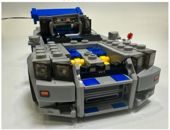
Remove the shown parts on the side, then put the wire with USB cable in between the studs
