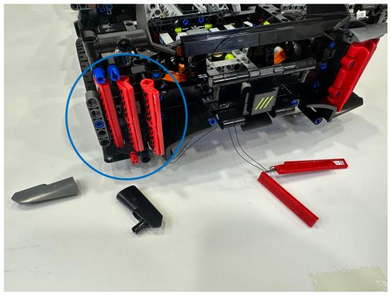
Remove the shown parts, move the remain lighting tiles to the left and assemble them
