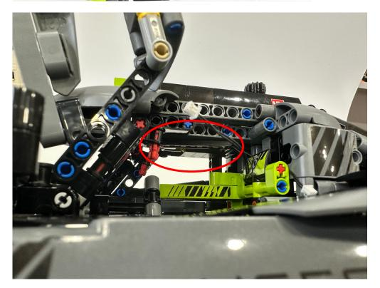
To power by USB, connect the USB cable with the connectors at the bottom of the car
