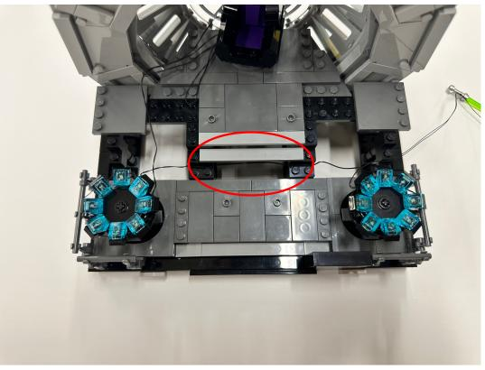
The connector will be moved to the back of the whole model, there's space at the back to make the wire get through
