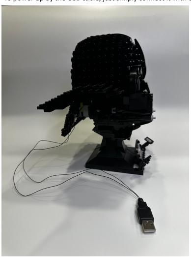
To power by battery, remove the back part from the helmet and stick the battery case as shown
