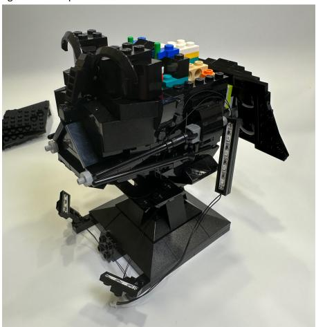
The cable from the spot light to lighting plate could be stabilized at the shown area Remove the shown parts, put the cable in between then put it back
