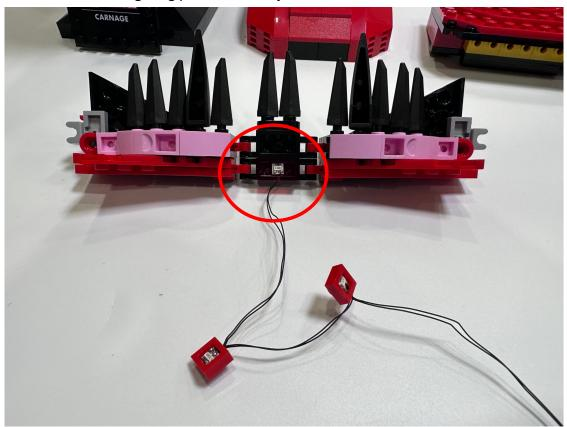
Then assemble the 1x1 lighting plates at the shown area of the jaw
