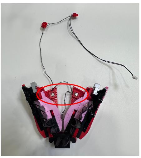
Restore the jaw, move the remain lighting plates to the top and the wires could be hidden behind the teeth at the red circle area
