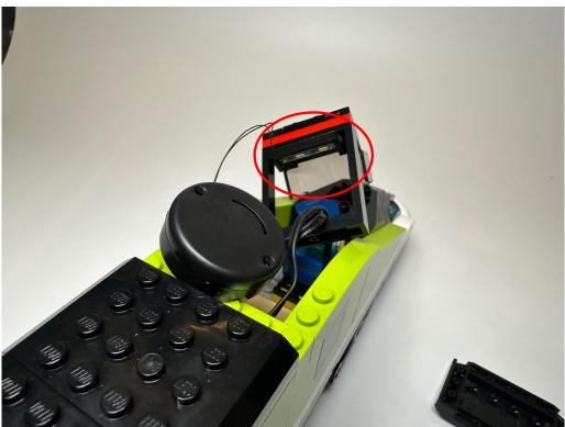
After that hide the battery case inside the train and restore the cover
