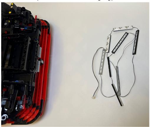
Stick the lighting tiles at the shown position and make sure the tile with connector attached belongs to the front side
