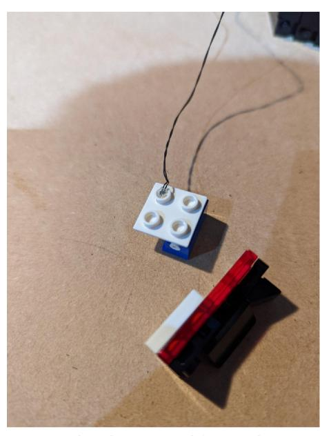
Place the bare led into the open stud.
