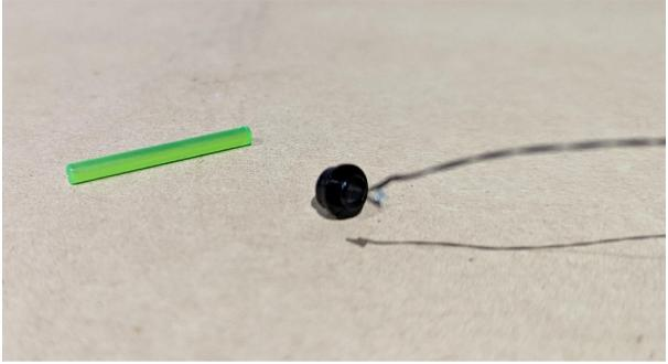
Bend the end of the bare green LEDs into a little hook. Insert it from the top of the included black open holed 1x1 round plate. It does not need to be inserted very far. Then insert the green bar into the top of the round plate. Repeat for all 4 green bars.
