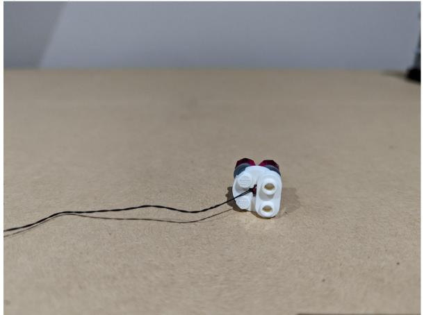
Put the bare red LED into the axle hole, ensure the wire runs between the two studs as shown before placing the plate on top. Put it back onto the ship.
