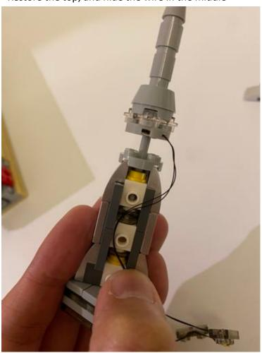
For the bottom, remove the 4pcs of 1x2 plates and replaced by the lighting parts, be sure the wire face outward
