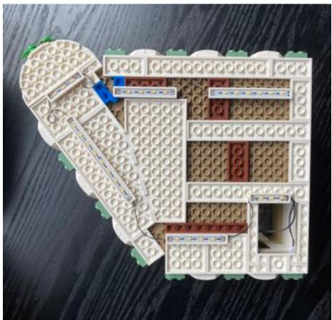
There would be 2 connectors, pull the longer one through the hole in purpose to connect with the roof ceiling lights
