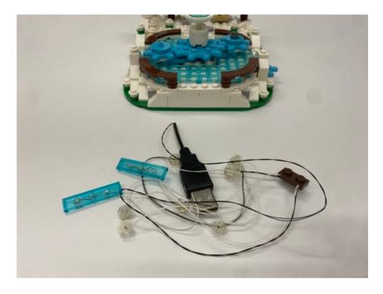
First, turn around the model then assemble the brown 1x2 lighting plate and replace the clear round brick for the lamppost
