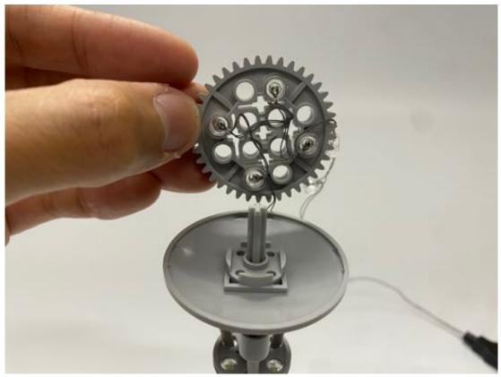
Restore the gear, then install the 4pcs of lighting round plates on top
