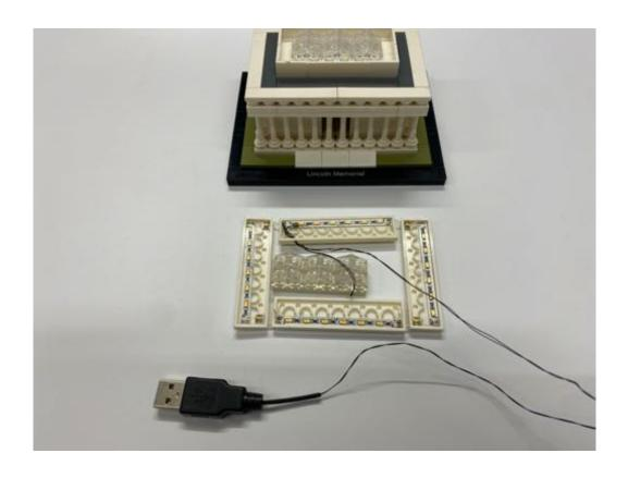
Start from removing the top, split it and remove the 4pcs of 2x8 plates and the top 2x8 plate with clear slopes attached
