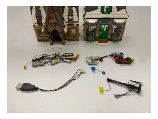
For the lamppost, just simply swap the round plate at bottom and the top parts to the lighting parts
