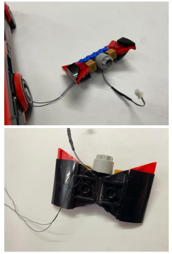
Put the part back to the car then pull the connector to the bottom
