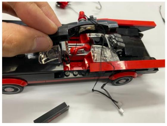
Then restore all the parts and pull the connectors out of the car
