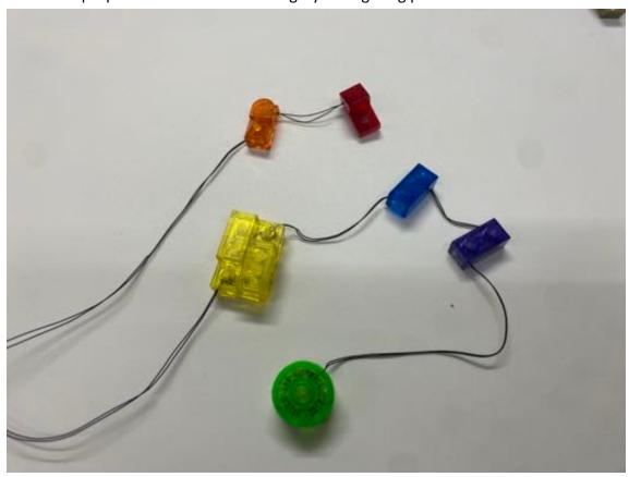
Start by installing orange and red, take the gold 1x2 plate, install the lights then put the gold plate back to cover the wire
