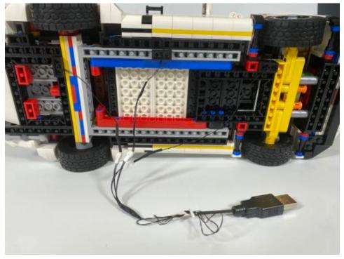
If powered by battery, connect to the battery case and stick it underneath the vehicle
