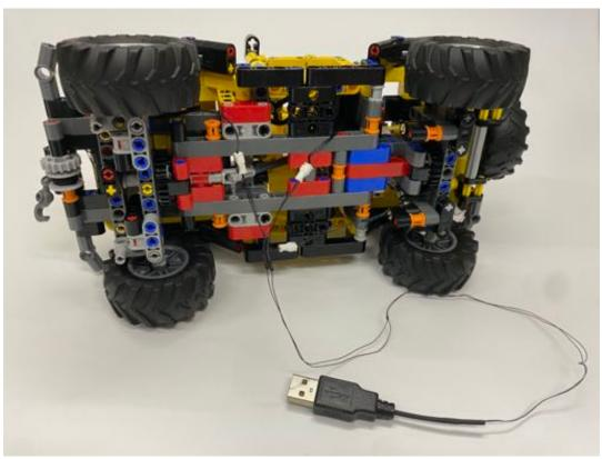
To power by battery, pull the connectors back to the passenger seat, connect with the battery case and place the case on the seat
