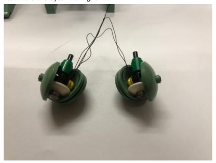
Assemble the eyes with lights back to the head, adjust the cables then put the cover back
