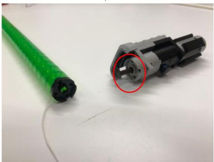
For the eye lighting parts, start by seperating the parts as shown
