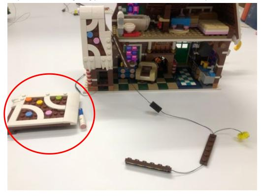
Pull the lighting parts to 2nd floor, to make it looks nicer you can hide cable as shown
