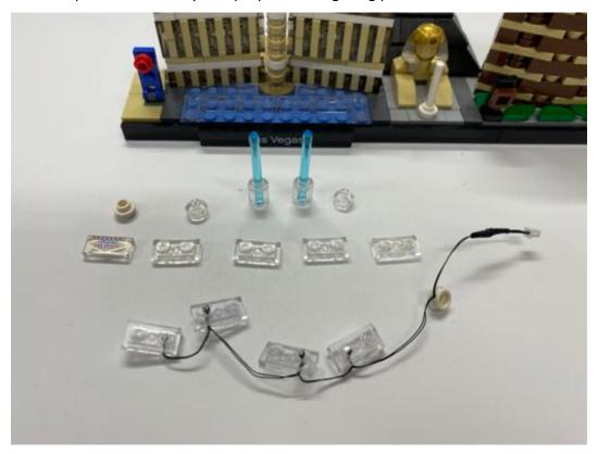
Replace the 1x2 plates and white round plate by the lighting part as shown, beware of the direction of the wires
