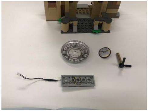
Install the light and connect the cables as shown and put the clock back on it
