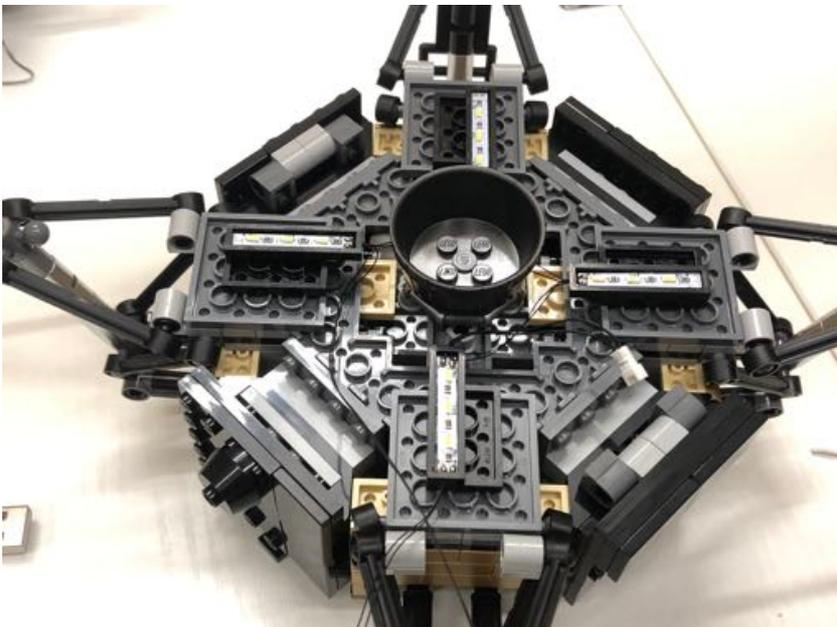
Pass 4 1x1 lights parts from the bottom thru the middle space
