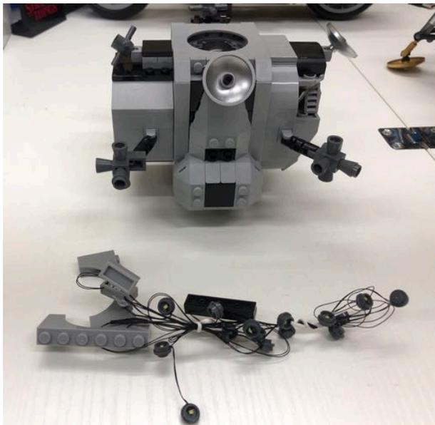
Remove 2 grey arches from the top and separate front and rear big parts as shown
